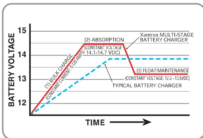
The Bulk Charge Voltage of typical liquid electrolyte lead acid batteries should be about 14.6 VDC. There is no one correct voltage for all types of batteries. Incorrect voltages will limit battery performance and useful life. Check the battery manufacturer's recommendations.
