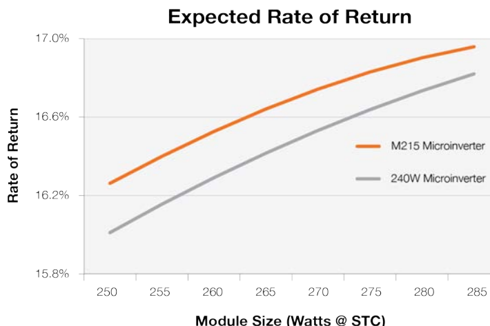
Figure 6: Expected rate of return is shown for different module and microinverter sizes.
