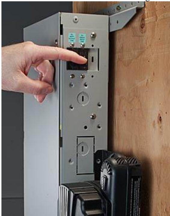
11. Remove the four screws holding the front cover of the Classic charge controller. **Do not let the front cover hang by the cable.**
