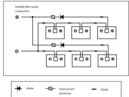
Fig. 14 Schematic diagram of electrical connection
