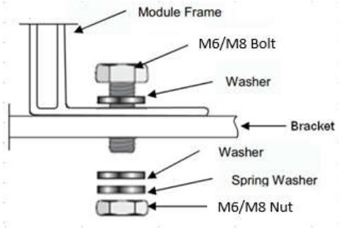
Fig. 7 Diagram of the bolt installation process
