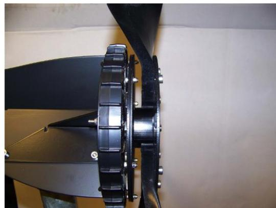
**Check the blade rotation-** Once the blades have been fitted and secured to the chassis, ensure that they rotate freely. Also take this opportunity to check that all of the blade and hub mounting screws are secure. Remember that the blades are SHARP!
