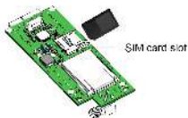
Figure 9: Inserting the card into the GSM modem
